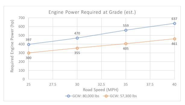
Figure 9: Estimated engine power required to sustain at a 6% grade
