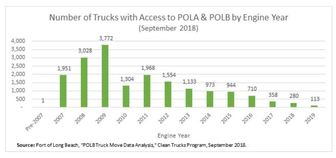
Figure 1. San Pedro Bay Ports drayage truck fleet constitution by engine model year
