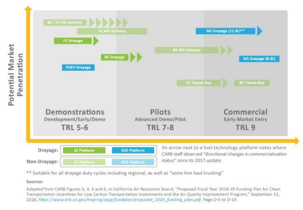
Figure 6. Summary of CARB's draft TRL ratings (NASA scale) for ZE and NZE HDV platforms
