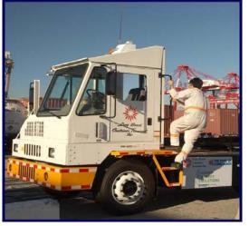
performance specifications. The LNG engine specified for the demonstration was the model year 2005 Cummins C Gas Plus 8.3 liter natural gas engine, rated at 250 hp and certified to the CARB on-road Optional NO<sub>x</sub> standard of 1.8 g/bhp-hr.
