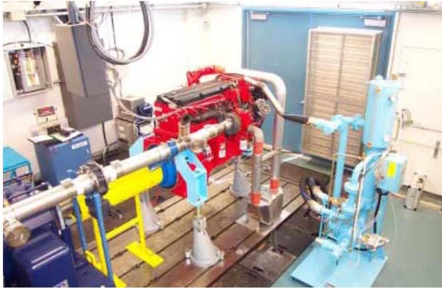
Figure 2.12: Westport GX Engine Undergoing Emissions Certification Testing
