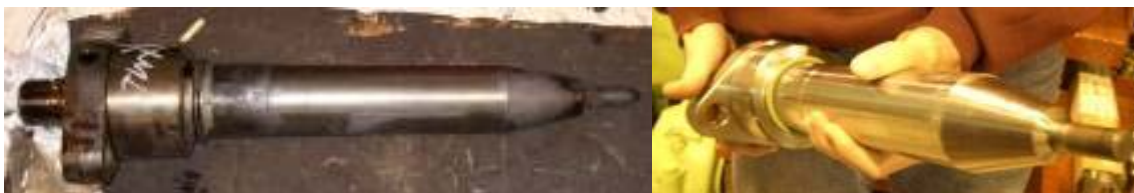
Figure 2.2: Conventional “Mini-Sac” Injector (left) Compared to the Slide Valve (right)
