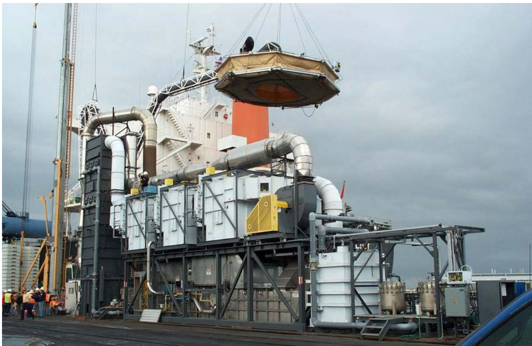
Figure 2.3: AMECS Emission Treatment System Installed Dockside
