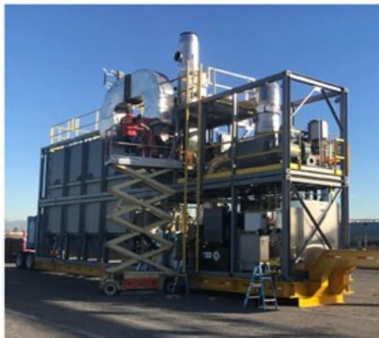
Figure 6: ShoreKat At-Berth Emissions Control System
