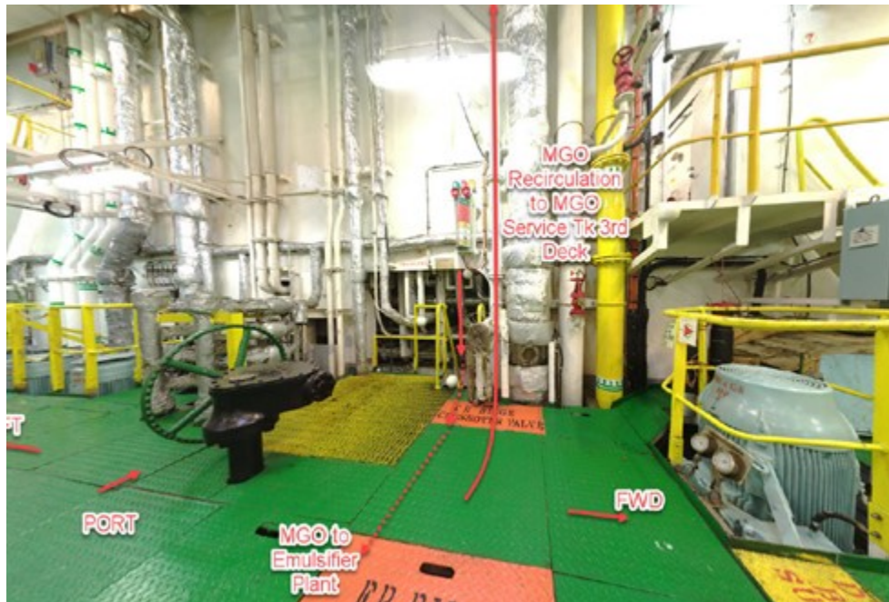
Figure 11: Engine Room Layout for WiF Installation
