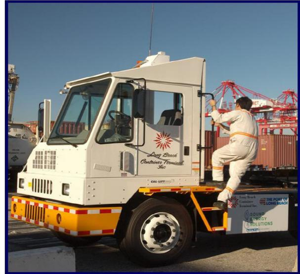
Phase 2 included operation of the LNG yard tractors at a marine terminal for a period of eight months. Demonstration commenced in June 2006 and was completed in January 2007. During this time, data were collected on the performance of the LNG yard tractors compared to a group of baseline diesel vehicles. Emissions testing was also conducted at the conclusion of the second phase;
