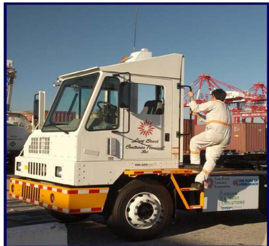
A total of three LNG yard tractors were deployed for performance testing and evaluation. Specifications for the LNG yard tractors were based on the Ottawa Commando 50 4x2 off-road terminal tractor performance specifications.
