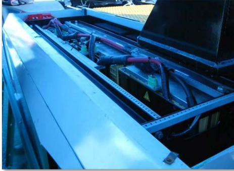
The lithium battery cells were assembled into the battery packs at Balqon's Harbor City, California facility and fitted with a proprietary battery management system (BMS) specifically designed for lithium-ion battery chemistry and characteristics. This TAP project also supported development of new charging algorithms to allow fast charge the lithium-ion batteries using the existing Balqon fast charger.
