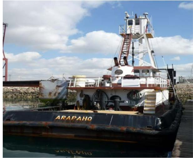
The Arapaho was repowered in late 2010 and is now equipped with two main propulsion 2010 Tier 2 MTU Detroit Diesel 12V 2000 M60 engines (805 hp, EPA engine family #AMDDN31.8MRR). As part of this TAP demonstration project, Hug will install and monitor two nauticlean® systems on each of the two Tier 2 main propulsion engines.
