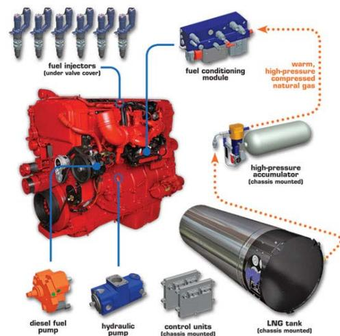
Simultaneously, a diesel fuel pump draws and pressurizes diesel fuel from its storage tank. Both the natural gas and diesel are then routed to a fuel conditioning module, where both fuels are pressure regulated, filtered, and sent to the fuel injector nozzles.
