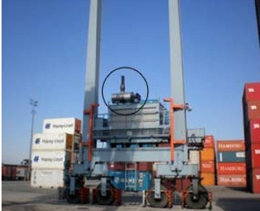
RYPOS redesigned and upgraded the HDPF/C™ for RTG cranes with an all-electric charged, active regeneration filter—the ActiveDPF/C™, and plans to do the same for top and side handler applications. The ActiveDPF/C™ is designed to regenerate at any exhaust temperature and is not affected by idle operation.
