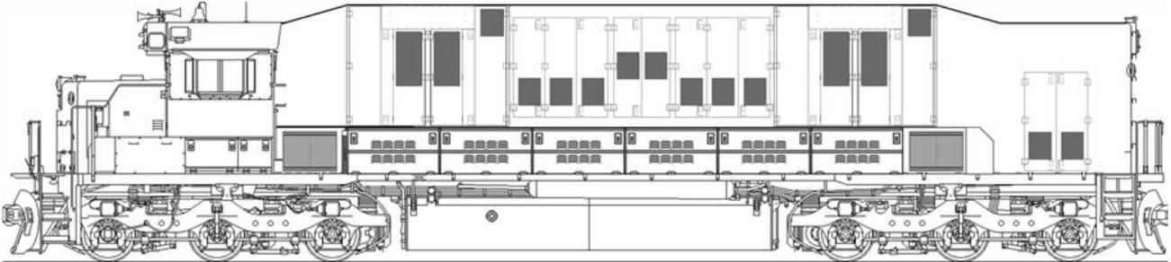
**Figure 6.6: VeRail VR21C4-df dual fuel locomotive showing location of CNG tanks above the frame, dual 1,200 HP near-zero emissions natural gas Power Modules (in yellow), and twin 600 HP Tier 4 diesel gensets (between the natural gas Power Modules).**
