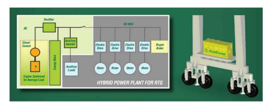
Figure 2.4: EcoCrane™ Hybrid Electric RTG Power System
