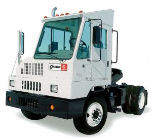
Yard hostlers (also known as yard tractors, terminal tractors, or utility tractor rigs) are common at port terminals, rail yards, and distribution centers. Their function is to move containers around the facility. At a port, containers are loaded off a ship onto a bobtail rig that is pulled by the yard hostler to an intermodal point or to a storage facility. Yard hostlers often sit idling as they wait in queues to pick up or drop off their loads.
