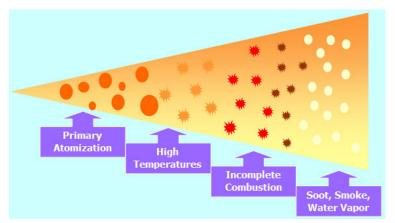
Figure 2.6: Combustion of Emulsified Biodiesel Fuel
