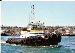
smaller displacement, Tier 2-certified third main engine positioned in the center of the tug and equipped with a selective catalytic reduction (SCR) exhaust treatment system. This configuration, named the ECO  $Tug^{TM}$ , will allow the majority of vessel operations to be performed using this single low emission center engine.
