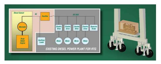
Figure 2.3: Conventional RTG Power System
