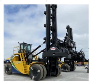
Figure 14: Zero-Emission Top Handler at Port of Oakland
