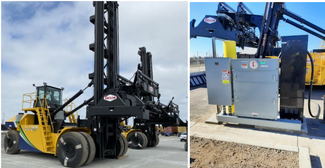
Figure 14: Zero-Emission Top Handler and Charger at Port of Oakland
