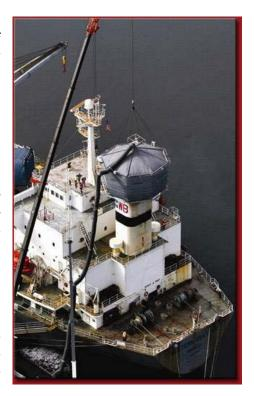
exhaust gases from escaping. The exhaust gases from the ship's auxiliary engines and the boilers were routed through a flexible duct to an Emission Treatment System (ETS) located on the dock adjacent to the vessel's berth. The ETS used multiple exhaust gas treatment technologies, including scrubbers and selective catalytic reduction, to remove both gaseous and particulate pollution.
