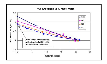
Figure 3: Changes in NOx Emissions with Changes in Fuel Composition
