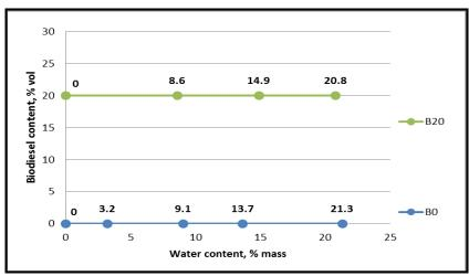
Note: Four fuels were tested without water (B0, B20, B50 and B100). The B0 and B20 fuels were also emulsified – the above diagram shows the water content of the emulsified fuels with B0 and B20. The values along the x-axis are the water content (% m)
