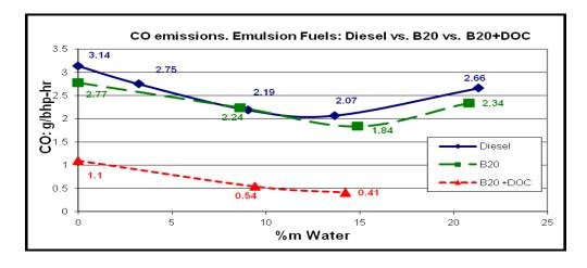
Figure 6 – CO Emissions – Effect of Fuel Composition and DOC
