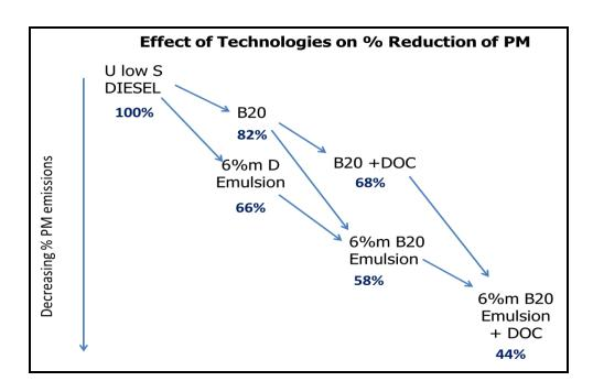
Figure 11: Effect of Emulsions, Biodiesel (B20) and DOC on PM Reductions
