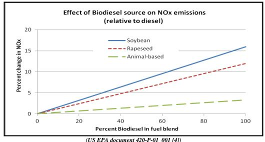
Note: On the x-axis the zero value represents the emissions from diesel alone; The 100% value represents % increase in emission with neat biodiesel.
