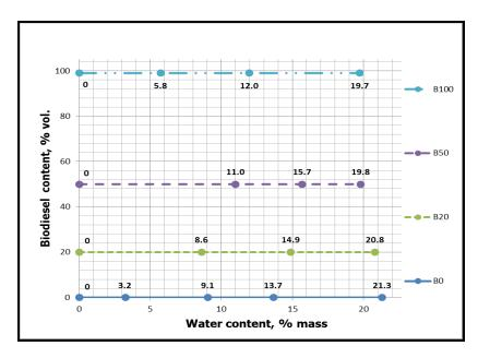
Note: The four horizontal lines are the four levels of biodiesel in the blend (0, 20, 50 and 100%v)
