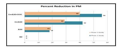
Figure 16: Reductions in PM by B20, EmB20 and EmB20+DOC Unit
