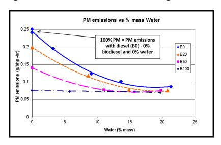
Figure 4: Changes in PM Emissions with Changes in Fuel Composition
