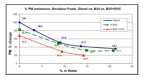
Figure 8 – PM Emissions – Effect of Fuel Composition and DOC
