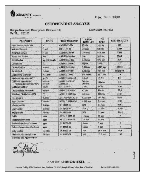
Table C.1: CoA for B99 Biodiesel fuel used to make B20 blend
