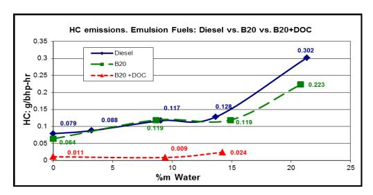
Figure 7 – Hydrocarbon Emissions – Effect of Fuel Composition and DOC
