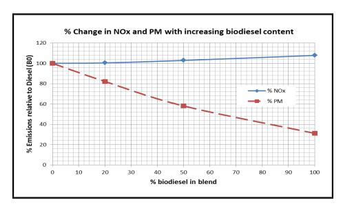
Figure 12: % Changes in NOx and PM Emissions vs. Biodiesel Content ~ Phase 1 Study
