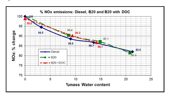
Figure 9: Percent NOx Reductions for B20, Diesel and DOC
