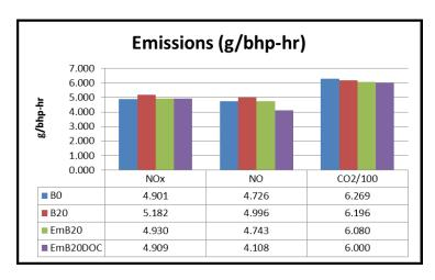
Figure 14: Emissions with B0 (diesel), B20, EmB20 and EmB20+DOC Unit
