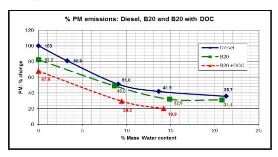
Figure 10: Percent PM Reductions for B20, Diesel and DOC
