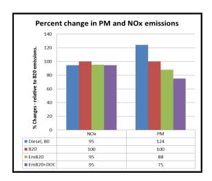
Figure 15: Relative Changes in PM and NOx Emissions (B20 = 100%)
