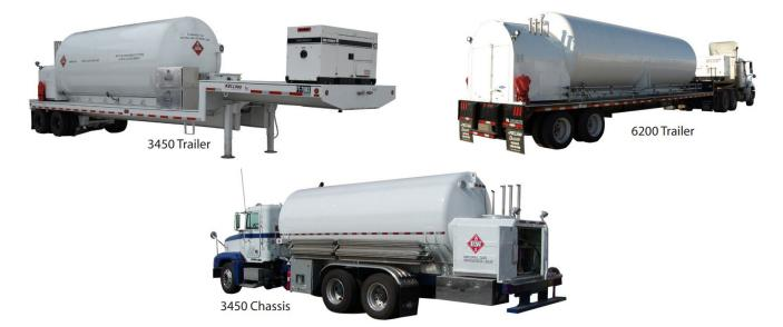
*Figure 21. Examples of mobile LNG fueling stations (photos from Chart Industries)*
