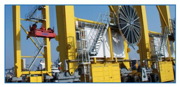
Figure 8. Cavotec ZE grid-electric conversion system for RTG cranes (courtesy of Cavotec)
