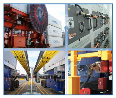
Figure 7. Conductix Wampfler ZE grid-electric conversion system for RTG cranes (courtesy of Conductix Wampfler)
