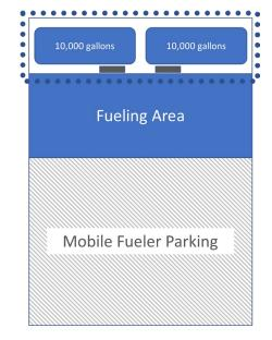
Figure 20. Example layout of an MTO's diesel fueling pad
