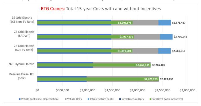
Figure 24. Total 15-year costs of ownership for the "Average RTG crane" scenario (NPV at 7% discount rate)
