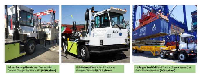
Figure 10. Three different ZE yard tractor demonstrations underway at multiple San Pedro Bay marine terminals
