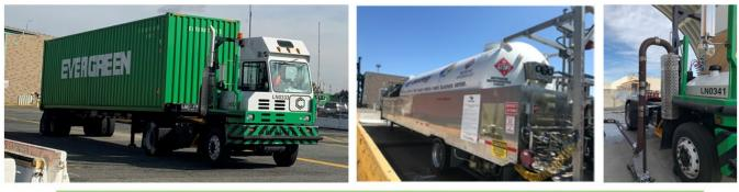
Left: NZE LNG-ICE yard tractor moving cargo at Everport (POLA); Center: Onsite LNG fueling station; Right: Emissions testing at UCR (photos by GNA)
