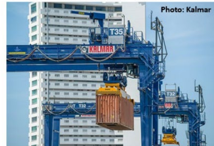
Kalmar NZE Hybrid-Electric RTG Crane
