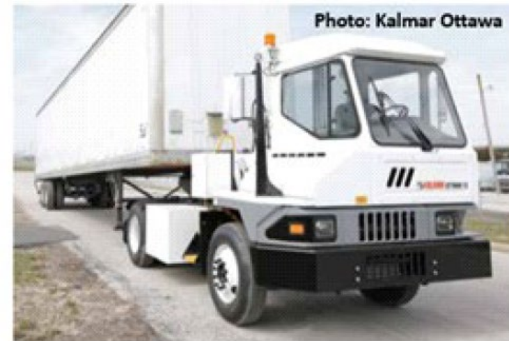
Kalmar Ottawa Battery-Electric Yard Tractor
