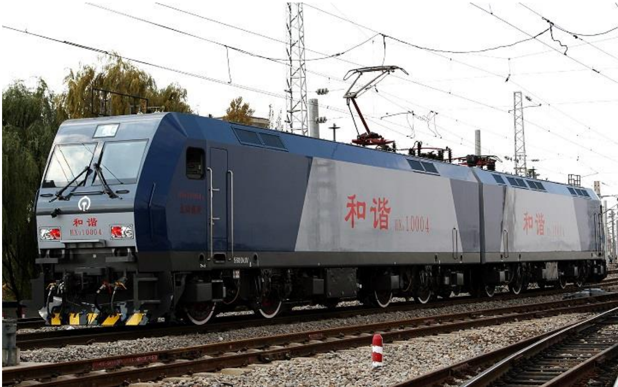
Fig. 5. China Railways HXD1 series freight locomotive set, under 25 kV overhead catenary wire (Photo: https://commons.wikimedia.org/wiki/File:HXD10004.jpg )
