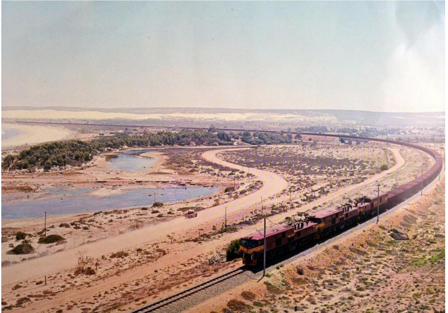
Fig. 4. South African Railways iron ore train on Sishen–Saldanha Orex line, pulled by electric locomotives under 50 kV catenary. (Photo: Peter Ball collection, http://www.theheritageportal.co.za/article/south-africas-world-record-breaking-train )
