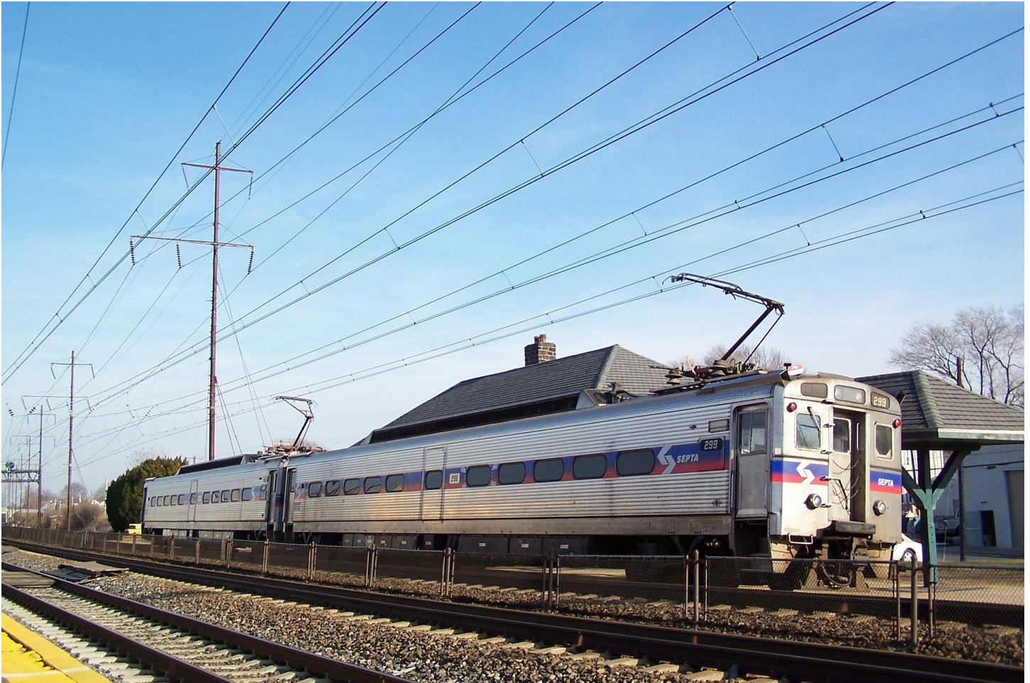
Fig. 11. SEPTA train on Northeast Corridor, under catenary supported by structures which also carry overhead transmission lines (Photo by jpmueller99, https://commons.wikimedia.org/w/index.php?curid=4007886 )
