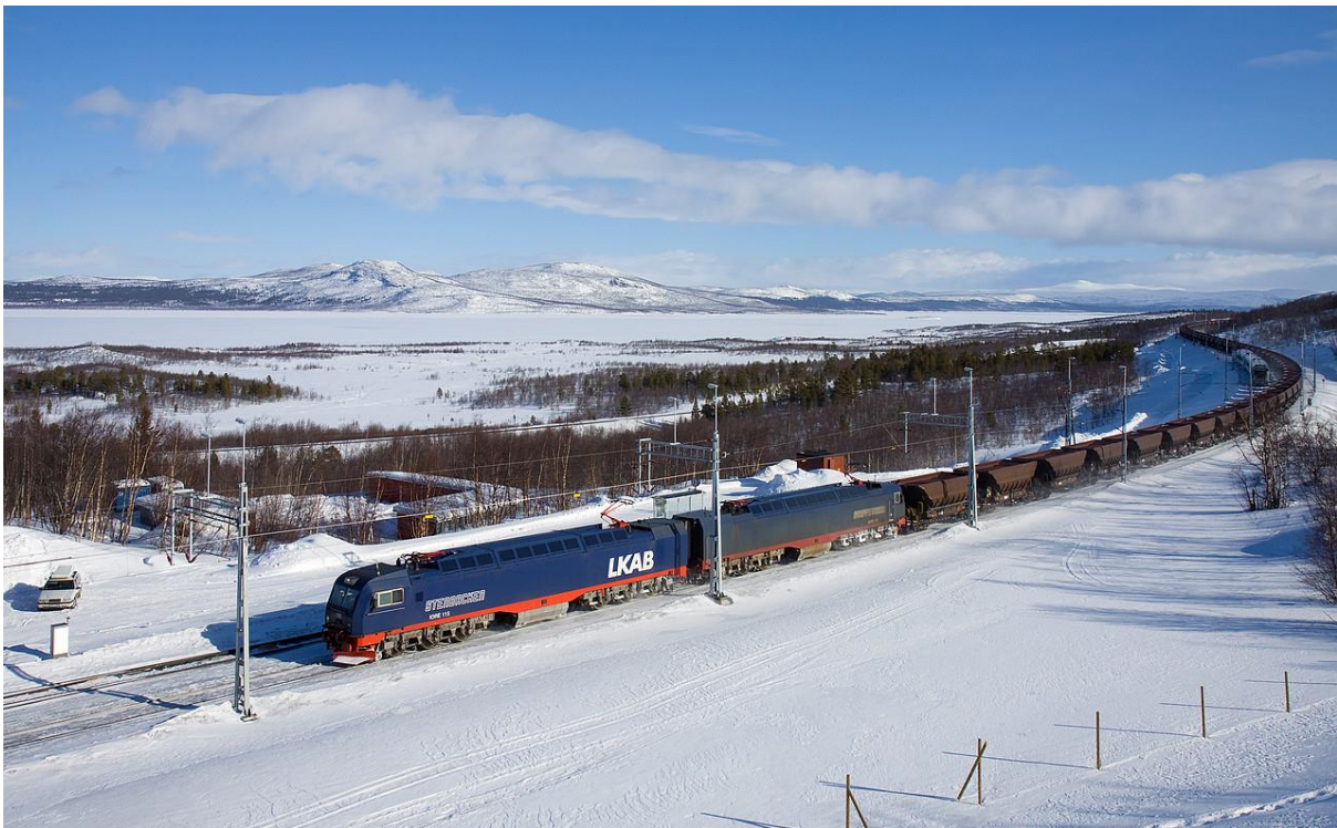
Fig. 6. Bombardier IORE electric locomotive set hauling an iron ore train between Sweden and Norway (Photo: David Gubler, 22.3.2011, http://bahnbilder.ch/picture/7743?title=iore )
