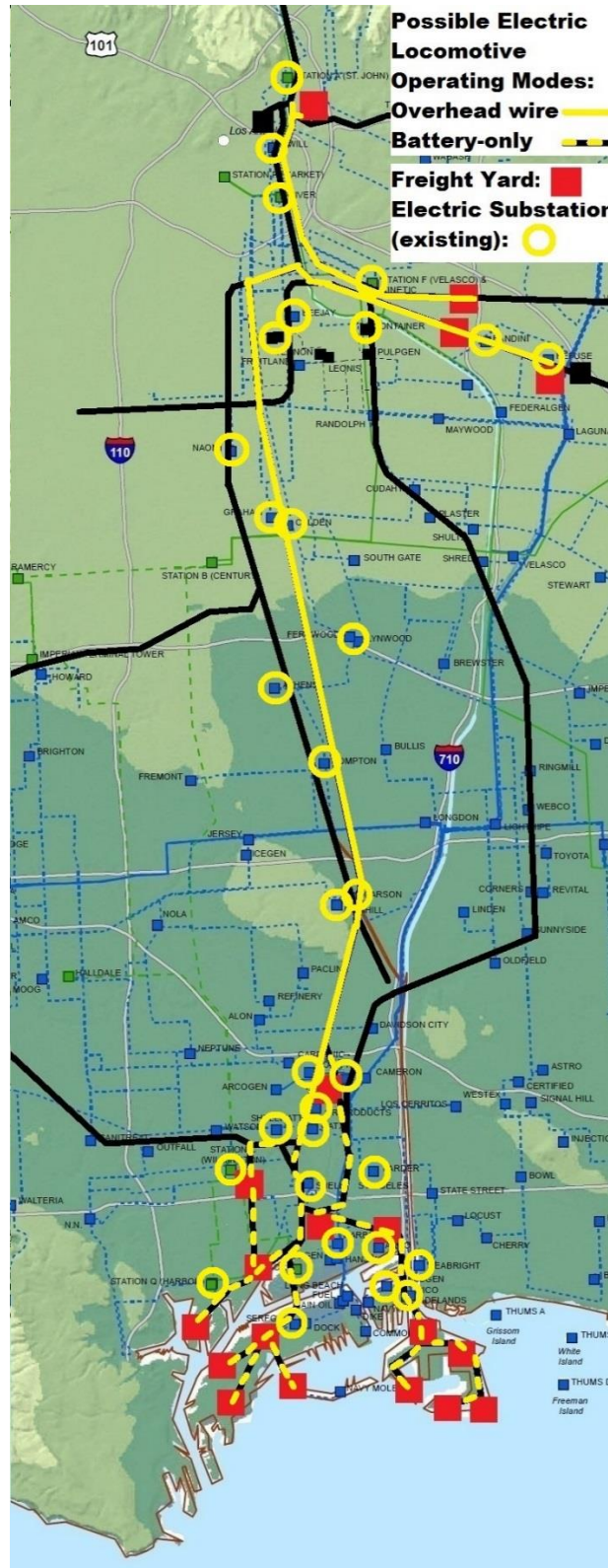
Fig. 16. Possible operating scenario of Alameda Corridor electrification using catenary/battery hybrid locomotives, overlaid on map of existing electric utility transmission lines and substations. (Background map: California Energy Commission)
