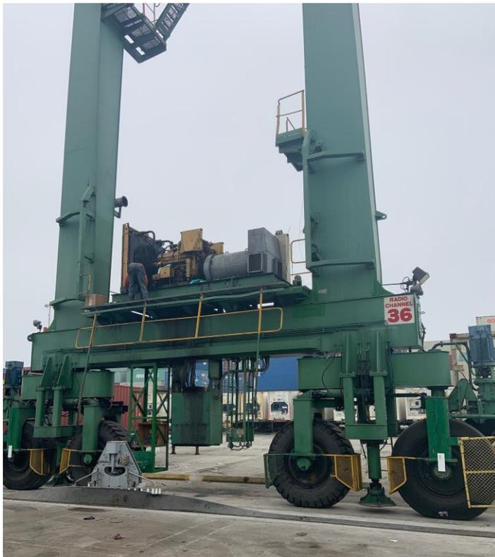
*Nine diesel RTGs are being repowered from diesel to full electric under the Zero Emissions Terminal Transition Project. See Section 5.17.*
