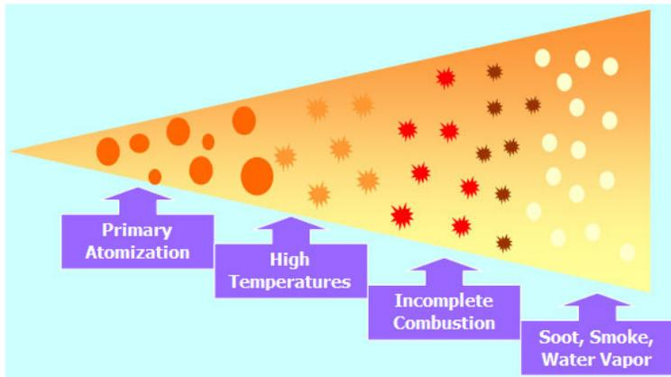
Unlike conventional diesel fuel, when emulsified fuel droplets are sprayed into the combustion chamber, they are atomized a second time as a result of the violent transformation of their water content into steam. This transformation of water into steam shatters the petroleum surrounding that water into much smaller droplets, shown in Figure 2.6 at left. Smaller droplets have a much greater
