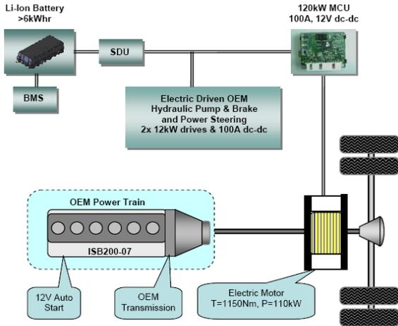
Three hybrid yard tractors will be integrated with hybrid drive systems and operate for a six-month period at LBCT at POLB. The hybrid vehicles will use a hybrid-electric drive system to combine the cleanest available diesel or alternative fuel engine technology with an electric motor, shown schematically in Figure 2.2.
