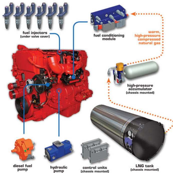
LNG fuel for the Westport GX engine is stored in the LNG tank mounted to the chassis of the vehicle. The liquid natural gas is drawn from the tank using a proprietary LNG pump that is powered by an engine-driven hydraulic pump. The LNG is then vaporized using excess heat from the engine's coolant system.
