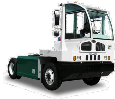
This follow-on TAP project will evaluate and demonstrate a lithium-ion battery as a technological upgrade to the lead-acid battery pack used in the previous TAP demonstration. The advanced technology lithium-ion batteries will more than double the vehicle range without adding additional weight.
