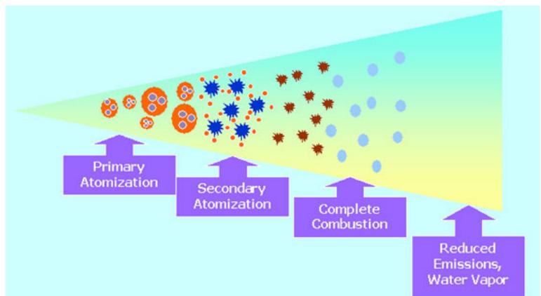
Since only the surface of each fuel droplet exposed to air can burn, larger liquid fuel droplets do not burn completely, leaving unburned carbon to collect on the surfaces of a combustion chamber or escape as PM in exhaust gases. This reduces overall thermal efficiency and increases harmful emissions, as denoted in Figure 2.6.
