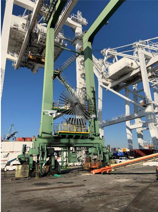
*Nine diesel RTGs are being repowered at SSA, Pier J from diesel to full electric under the Zero Emissions Terminal Transition Project. See Section 5.16.*
