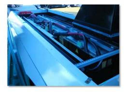
The lithium battery cells were assembled into the battery packs at Balqon's Harbor City, California facility and fitted with a proprietary battery management system (BMS) specifically designed for lithium-ion battery chemistry and characteristics. This TAP project also supported development of new charging algorithms to allow fast charge the lithium-ion batteries using the existing Balqon fast charger. Vehicle range tests were conducted using both dynamometer and field test
