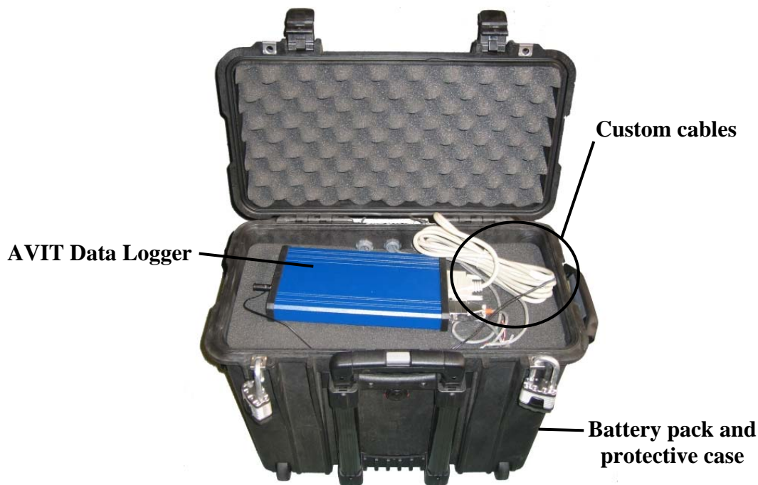
Figure 2. AVIT Data Logger with Added Equipment
