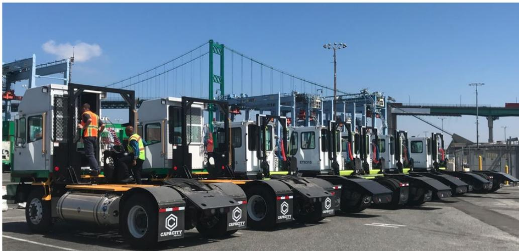
Figure 12. Two NZE LNG (left) and five ZE BE yard tractors undergoing prep for testing at Everport POLA (photo: GNA)
