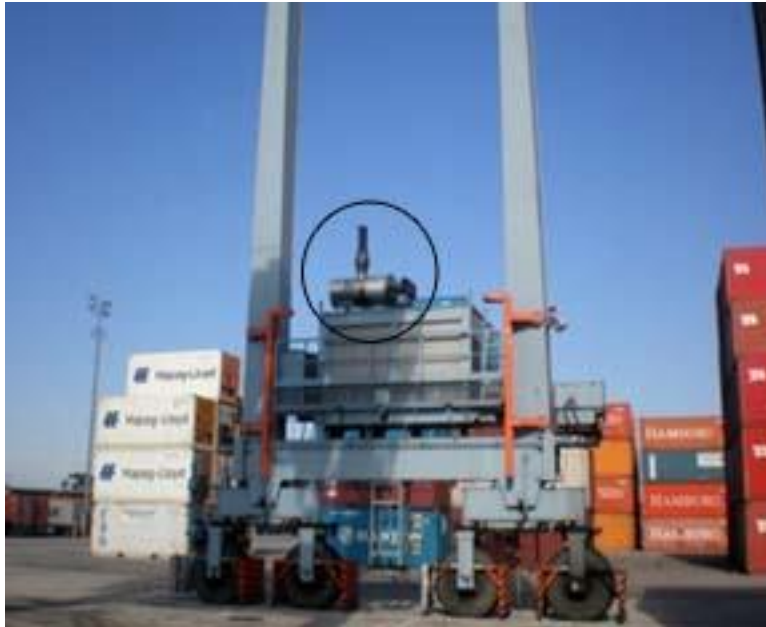
Figure 2.3-2: The RYPOS HDPF/C™ System Installed on an RTG Crane
