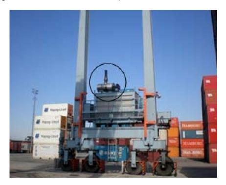
Figure 2.8: The RYPOS HDPF/C™ System Installed on an RTG Crane
