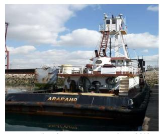
The Arapaho was repowered in late 2010 and is now equipped with two main propulsion 2010 Tier 2 MTU Detroit Diesel 12V 2000 M60 engines (805 hp, EPA engine family #AMDDN31.8MRR). As part of this TAP demonstration project, Hug will install and monitor two nauticlean® systems on each of the two Tier 2 main propulsion engines.
