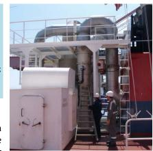
filter particulate contaminants from the ship exhaust stream before the exhaust is emitted to the atmosphere.
