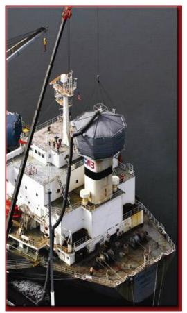
The **Pre-Conditioning Chamber**, which uses a counter-flow spray system to remove PM and water soluble organic gases. The spray water is treated with sodium hydroxide to simultaneously remove sulfur oxide pollution. The water spray also cools the exhaust gas, allowing smaller particles to coalesce such that they are more efficiently captured in subsequent phases of exhaust gas treatment;
