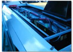
The lithium battery cells were assembled into the battery packs at Balqon's Harbor City, California facility and fitted with a proprietary battery management system (BMS) specifically designed for lithium-ion battery chemistry and characteristics. This TAP project also supported development of new charging algorithms to allow fast charge the lithium-ion batteries using the existing Balqon fast charger.
