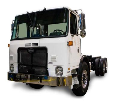
truck chassis manufacturers are offering vehicles equipped with the ISL G in a compressed natural gas configuration. The 8.9L engine is marketed as meeting 2010 US EPA and CARB emission standards. In addition, the relatively low cost of CNG, as compared to diesel fuel, makes this engine an attractive option for port drayage operators.
