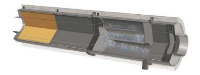
The Hug nauticlean® system utilizes passive regeneration, where particulate matter is continually burned off during vessel operation using a combination of the exhaust heat and a catalyst to facilitate combustion of the soot.
