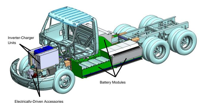
Figure 2.9: Overall Layout of Electric Drayage Truck Design
