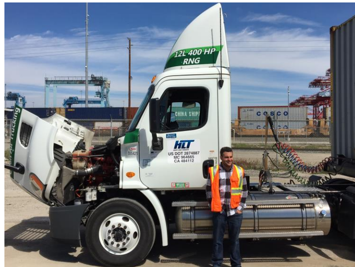
Figure 3 Near-Zero Emissions (NZE) Natural Gas Truck
