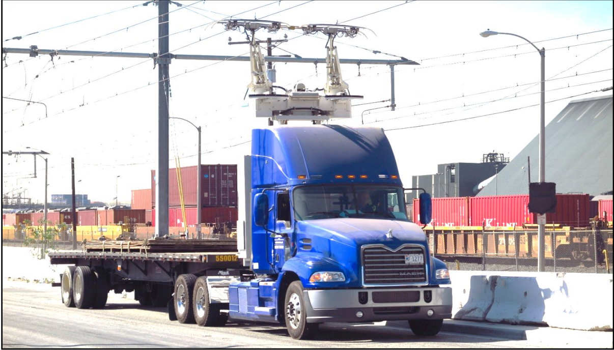
Figure 6: Demonstration of the Overhead Catenary System
