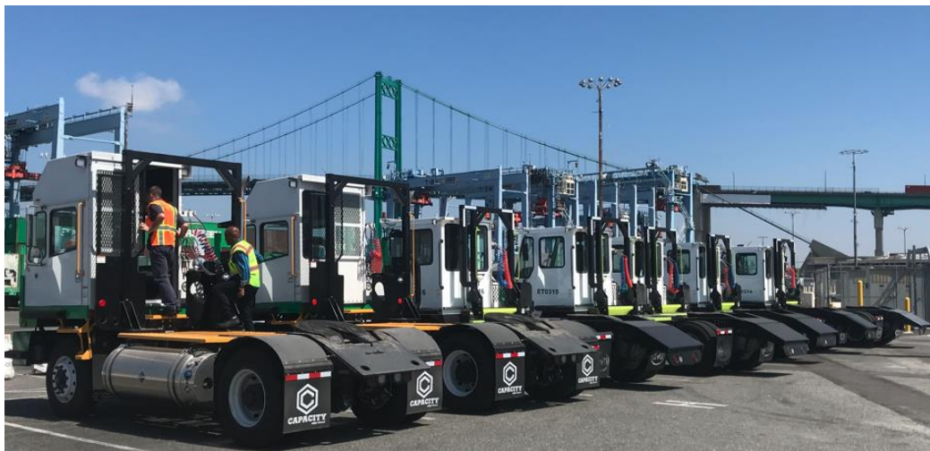
Figure 12. Two NZE LNG (left) and five ZE BE yard tractors undergoing prep for testing at Everport POLA (photo: GNA)
