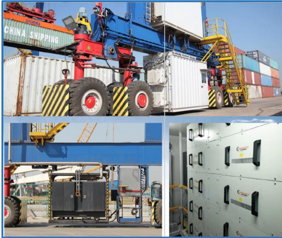
Figure 6. Conductix-Wampfler NZE hybrid-electric conversion system for RTG cranes (courtesy of Conductix-Wampfler)
