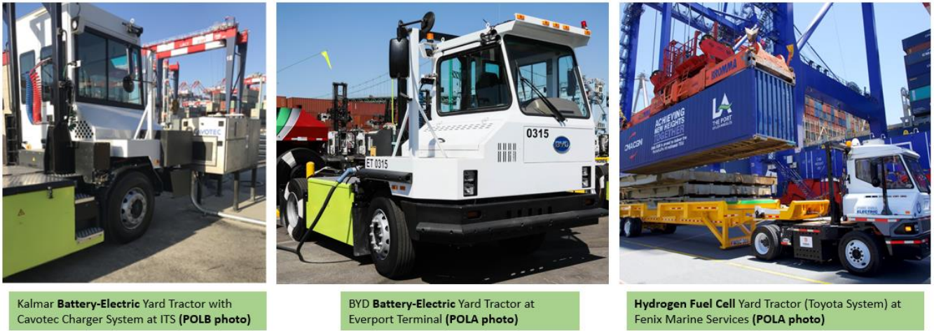
Figure 10. Three different ZE yard tractor demonstrations underway at multiple San Pedro Bay marine terminals
