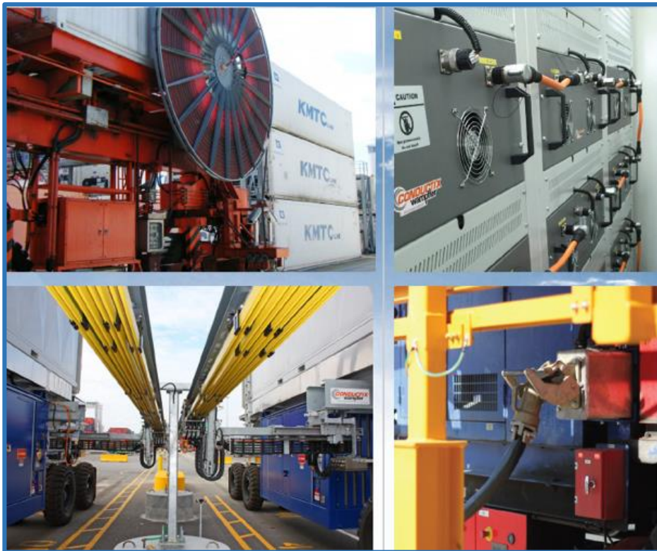
Figure 7. Conductix Wampfler ZE grid-electric conversion system for RTG cranes (courtesy of Conductix Wampfler)
