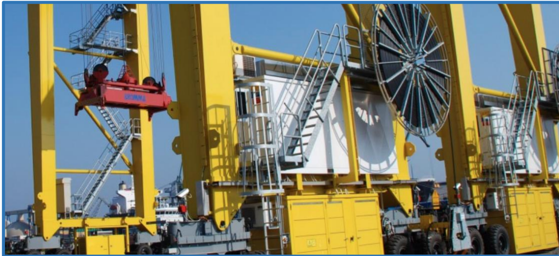
Figure 8. Cavotec ZE grid-electric conversion system for RTG cranes (courtesy of Cavotec)
