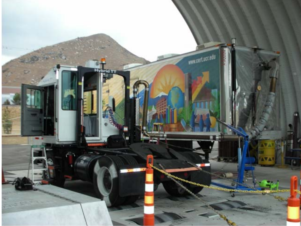
Figure 3-4 Figure Showing the UCR HDD Chassis Dyno with YT and MEL
