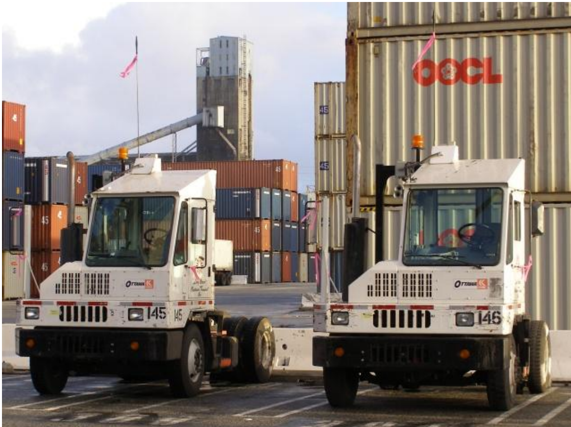
Figure 1 - Yard hostler vehicles at Port of Long Beach utilized during data logging.
