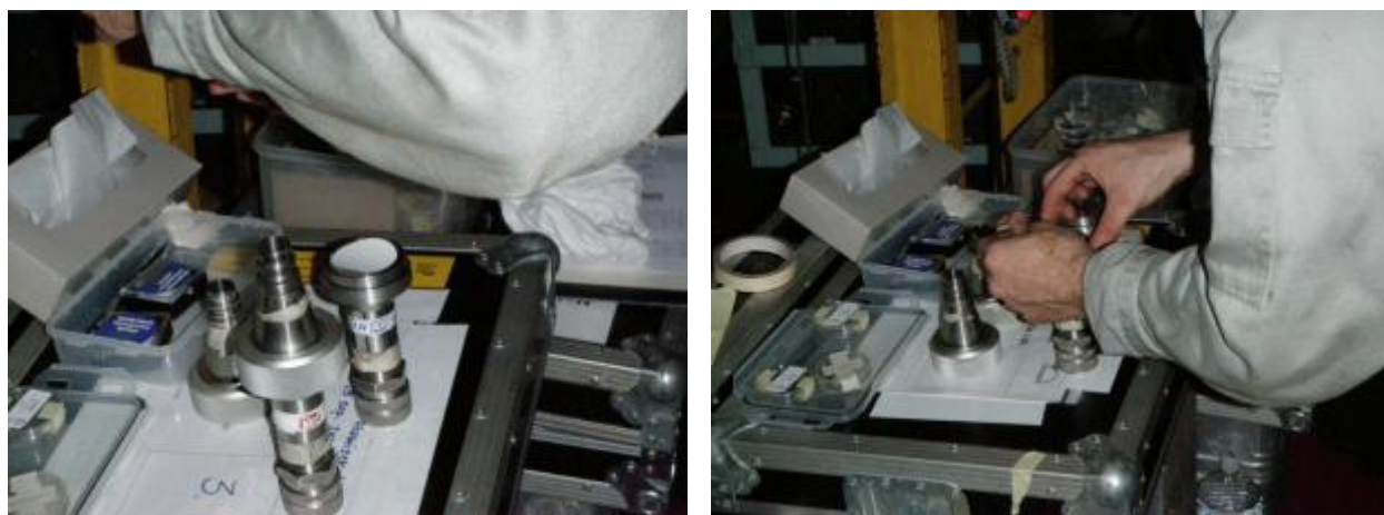
Figure 3.3: MDT Technician Prepares Particulate Filters in Preparation for Sampling in Accordance with ISO 8178
