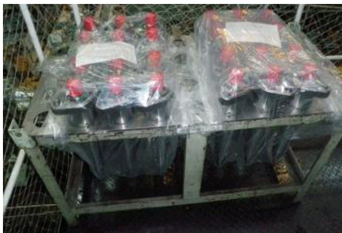
Figure 2.3: Conventional (C3) Nozzle and Low-NO x Conventional (C11) Nozzle Fuel Valves Prior to Installation and Testing.
